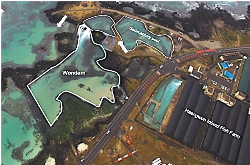
Figure 2. A close aerial view of Haengwon Inland fish farm and the Wondam. The large inland fish farm complex dumps its emission into the sedimentary pool, and then the emission is filtered out to the Wondam. (Photo taken by a drone)
