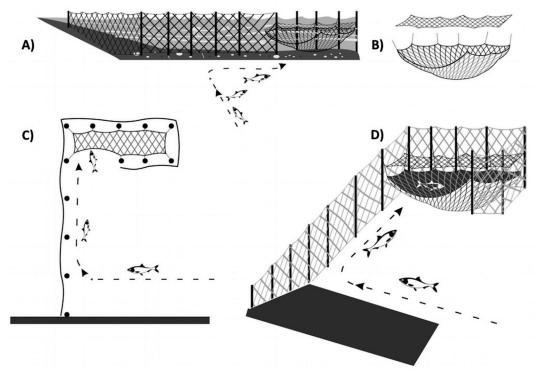
**Figure 2.** Design of the dalyan fishing gear: (A) Side view of poles, leader, and trap—Fish swim perpendicular to the shore, reaching the leader, which leads them to the trap; (B) Side view of the trap—The fish fall into the lower net of the trap, and fishermen in their boats gradually take them out; (C) Top view of leader and trap; and (D) View from the shore of the fish swimming towards the leader, which then leads them to the trap. Schematic dalyan created by Bozhidar Manolov.
