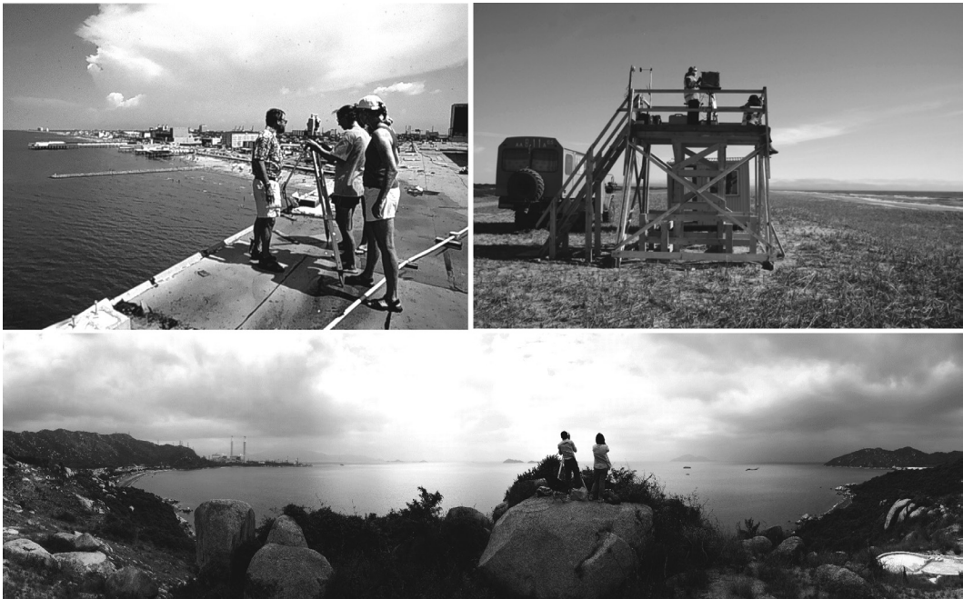
Figure 1. Examples of diversity in theodolite station platforms: Top left: Bernd Würsig and Texas A&M University graduate students tracking common bottlenose dolphins ( Tursiops truncatus ) off Galveston, Texas, in the 1990s from a hotel rooftop (32 m). Top right: Olga Sychenko tracking western gray whales ( Eschrichtius robustus ) off Sakhalin Island, Russia, in 2010 from a specially constructed platform (8 m). Bottom: Mott MacDonald field team members tracking Indo-Pacific humpback dolphins ( Sousa chinensis ) off Hong Kong in 2015 from a naturally elevated landscape (51 m). Photos courtesy of Bernd Würsig, Glenn Gailey, and Heidi Yu, respectively, with permission.
