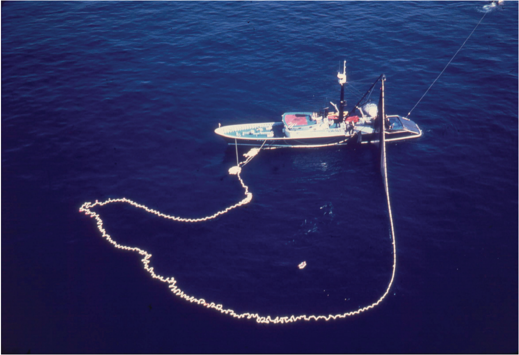
Purse-seine set on tuna associated with dolphins (Aerial photo by Wayne Perryman)
