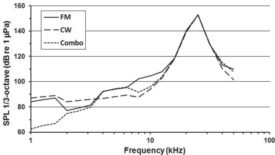
**Figure 4.** The  $1/3$ -octave spectra of the FM, CW, and Combo signals recorded in the pool (all three signals had similar spectra with peak frequencies at 25 kHz). The signals were recorded up to 50 kHz as this is the upper limit of the harbor seal's hearing frequency range (Kastelein et al., 2009a, 2009b).
