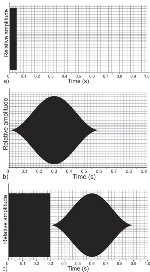
**Figure 3.** The waveforms of the three sonar signals of around 25 kHz used in the present study: (a) the 50-ms FM sound type, (b) the 600-ms CW sound type, and (c) the Combo sound type (300-ms FM followed by 600-ms CW); the duty cycles and inter-pulse intervals of the sequences that the harbor seals (*Phoca vitulina*) were exposed to in the study differed between the three sound types (see Table 1).
