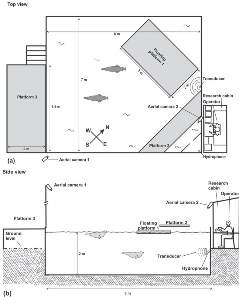
**Figure 1.** Top and side scale views of the study facility, showing the study animals, the location of the aerial cameras, the underwater transducer emitting the sonar signals, the listening hydrophone, and the three haul-out platforms. Also shown is the research cabin which housed the equipment and the operator.
