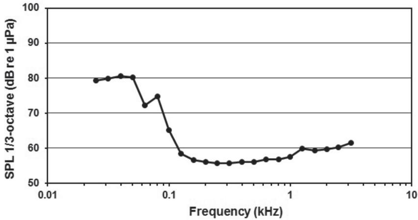
**Figure 2.** The background noise in the pool represented in  $\frac{1}{3}$ -octave bands (SPL averaged over 10 s). Above 3.5 kHz, the noise was dominated by the self-noise of the recording system.
