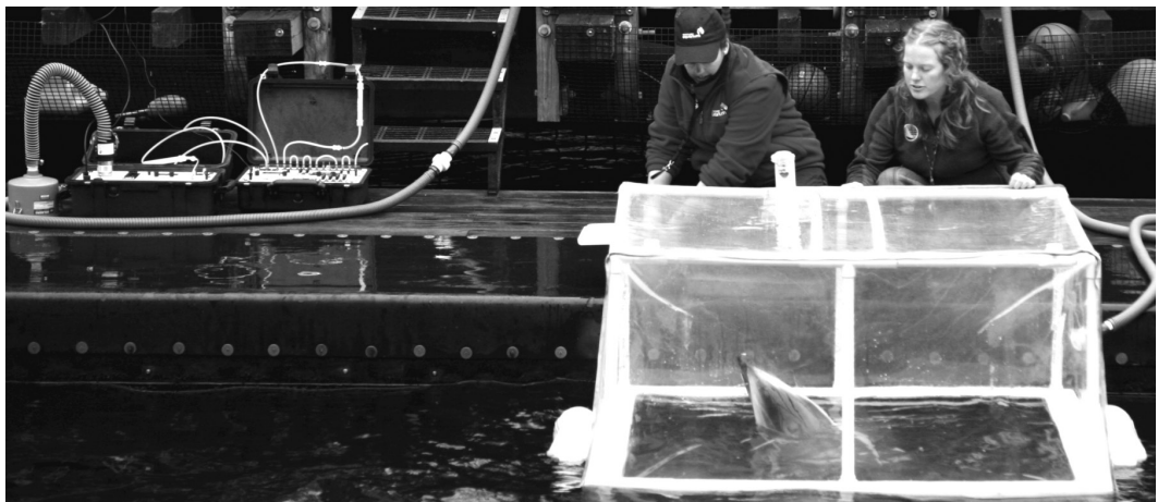
Figure 1. Experimental set-up shows Pacific white-sided dolphin F002 stationed under the floating respirometry dome. A vacuum hose runs from the dome to the mass flow pump (far right to far left of the photo), and the excurrent air flow is subsampled for gas concentrations (far left of the photo).
