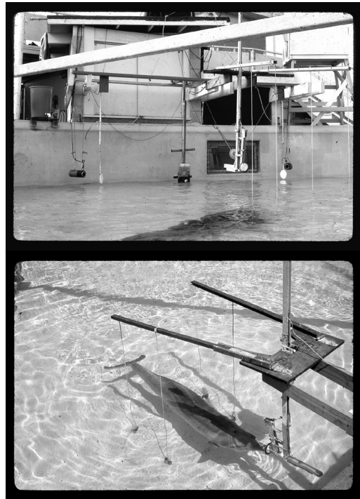
Figure 9. Top: View of initial apparatus used to test Kea's auditory learning and memory abilities; the water has been lowered for pool cleaning. The left and right J9 underwater speakers can be seen, each with a response paddle nearby. A channel of suspended ropes defines the "listening" area, with a "start" paddle at the channel's end. Just beyond the start paddle is a centrally located speaker that may play a "sample" sound. The two alternative sounds, one of them a "match," later appear at the J9 speakers, one at each speaker. Bottom: Kea enters the rope-channel listening area and presses the start paddle to begin a trial.
