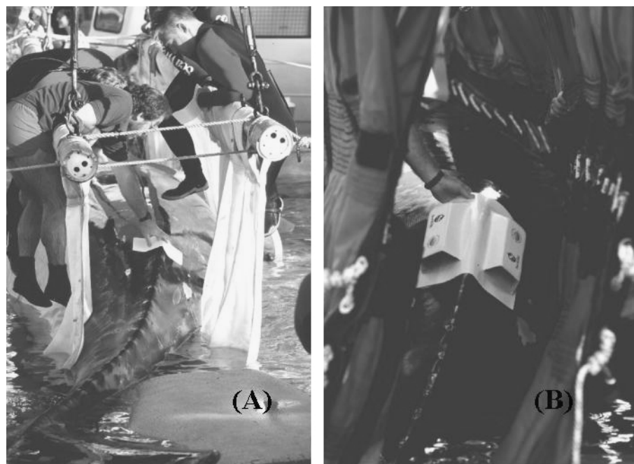
Figure 1. Custom-fitting housing for attachment of radio transmitters to a rehabilitating gray whale calf (JJ); A. creating the base mold shape; B. testing fit of final housing design.
