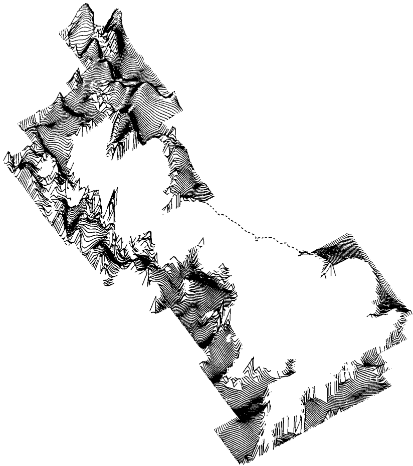
Figure 2. Local geomagnetic field for sea areas around the British Isles. Adapted from maps compiled by the Institute of Geological Sciences (1972) and displayed using the ASPEX computer graphics package. The land and areas outside the survey are shown as zero or datum. It is important to note that the land/sea border represents an artificial division as far as geomagnetic topography is concerned (see Figure 1). To display the topography on a single map, the data have been smoothed and truncated. No survey was available for the sea areas off the east coast. The angle of projection was chosen both to give an overall impression of the field and to illustrate as many as possible of the sites not shown in Figure 1.
